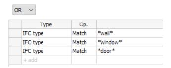
This selector finds the objects, which have in the IFC type field the text "wall", or "window", or "door". So in this case all walls, windows or doors will be selected of both types IfcWall and IfcWallStandardCase.
