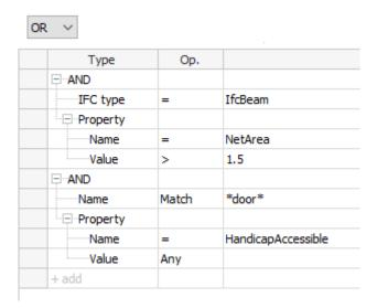
The above selector selects the objects, which are of the type IfcBeam, and consists of the property NetArea with the value greater than 1,5, or objects, which the name includes the text "door" and includes the property HandicapAccessible with any value.
